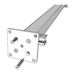
Remove screws on bottom of post that affix base plate to post
