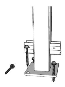
Re-affix post to deck with appropriate lag screws (not part of the ProBuilt railing system)
